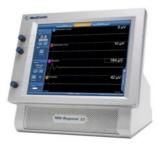
Intraoperative NIM nerve monitoring systems enable surgeons to identify, confirm, and monitor motor nerve function to help reduce the risk of nerve damage during various procedures, including ENT and general surgeries.
